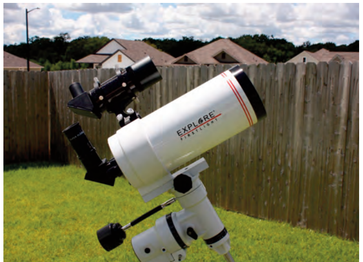
Image 12 – The 100 mm Mak-Cass shown with the author's 8x50 finder scope. A 1.25-inch diagonal with a 1.25-inch 25mm Plossl eyepiece are also shown attached to the telescope.
