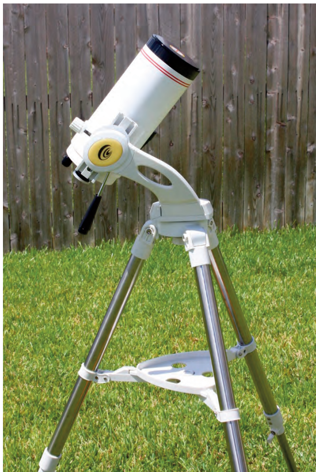
Image 4 – The Twilight Nano mount has one arm that received the dovetail plate screwed onto the telescope. This is an alt-azimuth mount.
