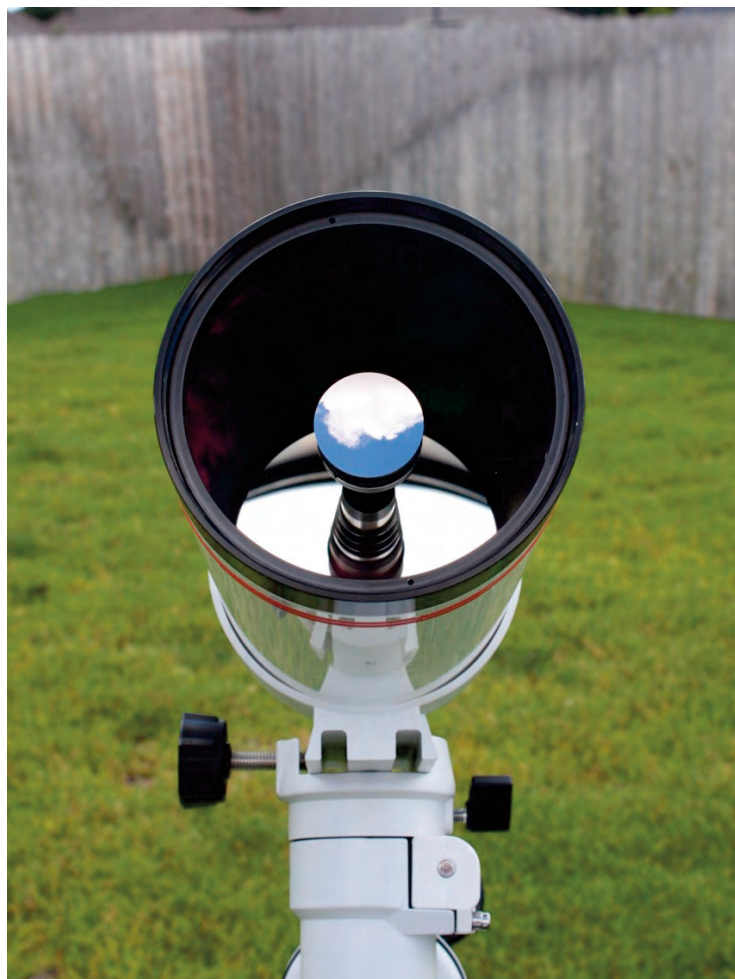
Image 13 – The telescopes optics are shown here. The corrector lens covering the tube opening holds the secondary mirror in place. The lens is so clean it is practically invisible in the image.
