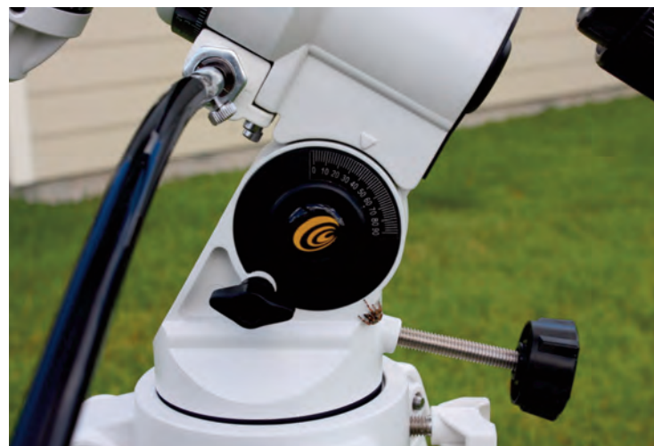
Image 8 – The hand-turn bolt on right is used to adjust the mount for the user's latitude. A latitude gauge appears on the side of the mount. There is a hand knob that must be loosened to adjust the latitude and tightened to hold it in place.
