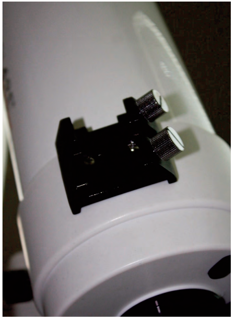
Image 10 – The author replaced the red-dot shoe with one that would hold a 6x30 or 8x50 finder scope.
