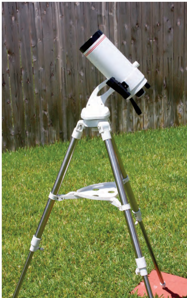
Image 3 - The Explore Scientific 100 mm f/14 Maksutov-Cassegrain telescope attached to a Explore Scientific Twilight Nano mount.
