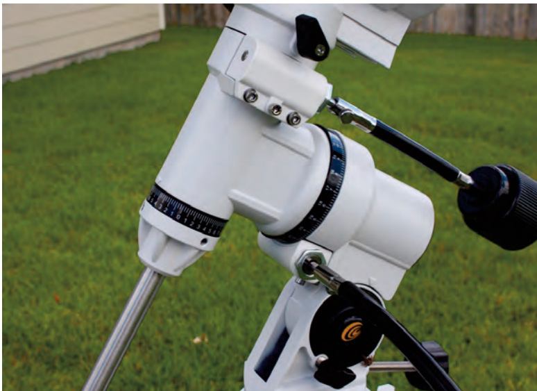
Image 6 - A close-up view of the EQ3 mount that arrived with the telescope. Note the setting circles on each axis as well as the slow motion hand knobs.
