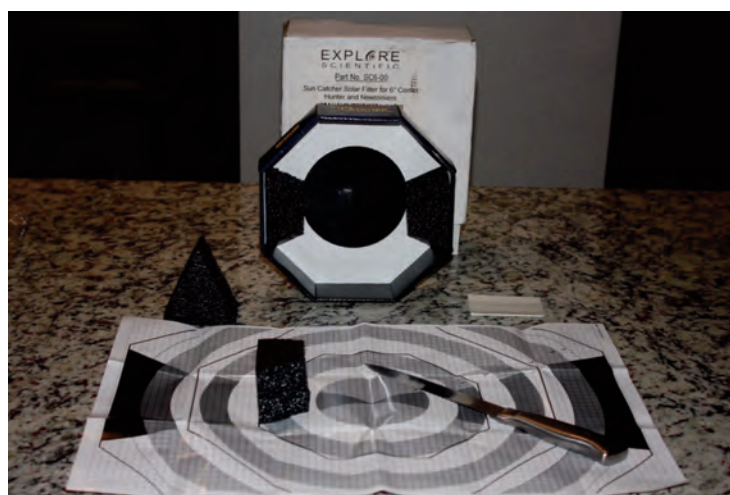
Image 14 – The Explore Scientific Sun Catcher Solar Filter can fit various diameter optical tube assemblies. A template is provided to cut out foam wedges to hold the filter on the various-diameter tubes.
