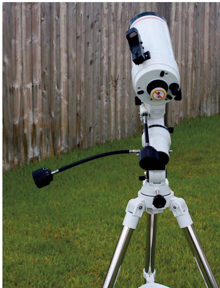
Image 7 – The red-dot finder atop the telescope came with the telescope. The focusing knob is on the back right side of the optical tube assembly.
