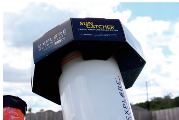
Image 16 – This view shows how the foam wedges glued onto the solar filter housing securely hold the filter onto the telescope.
