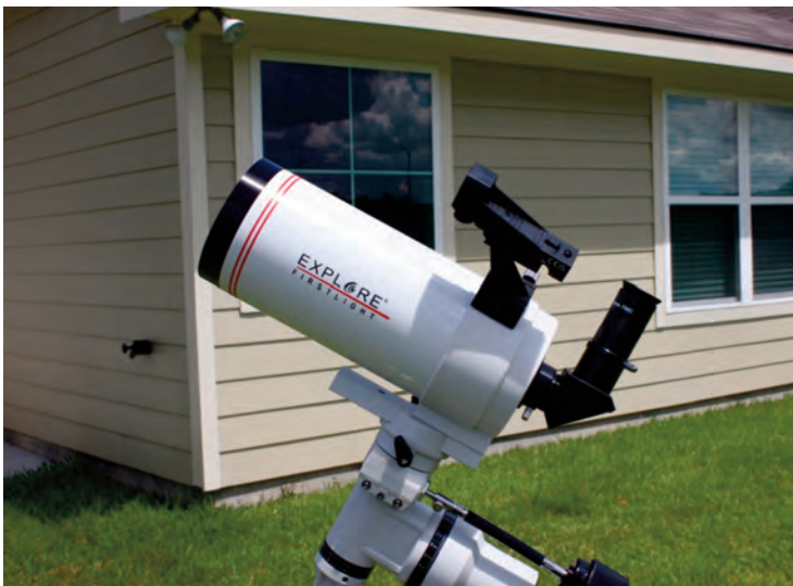
Image 11 – The author purchased a 3D printed bracket to hold the red-dot using the same shoe for his optical finder scopes.
