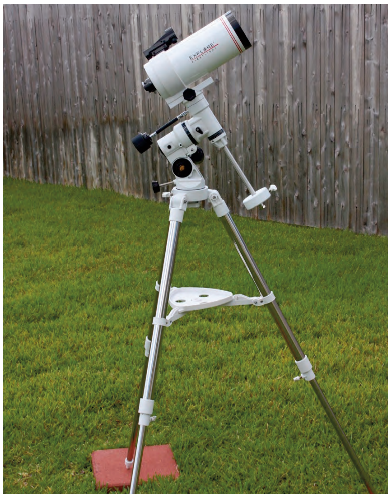
Image 5 - Here the 100 mm f/14 Maksutov-Cassegrain telescope is attached to an Explore Scientific EQ3 German equatorial mount.
